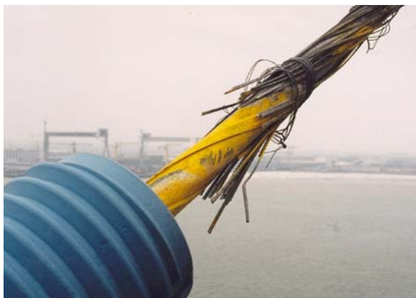
C - Fretting fatigue – frottements torons / colliers
